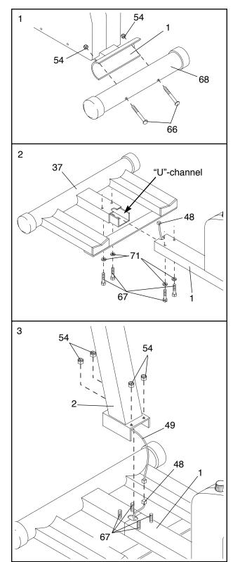
Slide the "U"-channel on the Rail Stabilizer (37) into the Base (1). Make sure that the Reed Switch Wire (48) is extending from the hole formed where the two parts meet; be careful not to damage the Reed Switch Wire.
